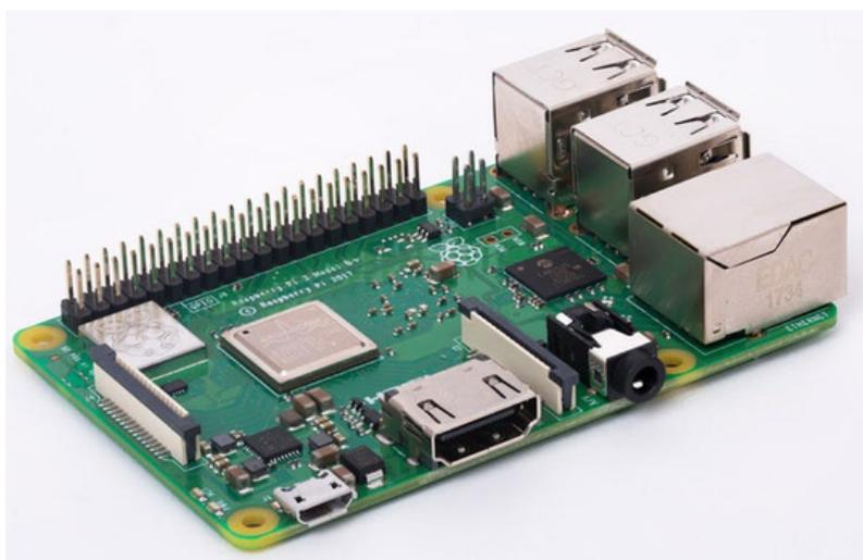
Figura 5 Raspberry Pi 3 Model B+
